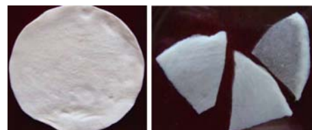
图 1 材料 ECM1-4 外观及在水中浸润后的形态 Fig. 1 Appearance of ECM1-4(left) and modality in water(right)
