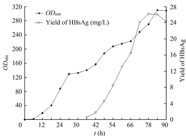
Fig. 6 Curves of the growth of the strains and expression of HBsAg in bioreactor
